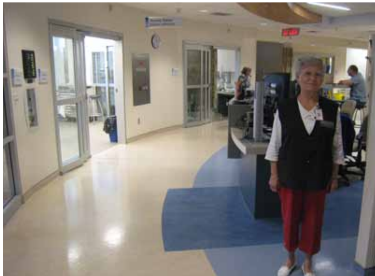
Peggy Richardson, Team Leader of ER volunteers, in the new Emergency Room at KDH. Note the curving hall, which allows nurses to see every patient bay from the nursing station.
